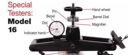
The Model 16 Tester is affixed to the stock piece by means of a chain clamp which can secure the tester frame to anything from about 4" thick up to 16" in diameter.
